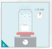
Put the open vial with inserted prosthetic restoration on the heater plate. Bring the VALLEOND<sup>TM</sup> solution to a boil and then leave it to boil for 5 minutes. When the solution becomes turbid, the coating synthesis is completed. Take the vial off the heater.
