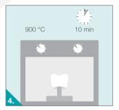
Put the coated prosthetic restoration into an oven. For best results use the following thermal treatment program: 900 °C / 1650°F, 10 min hold. After the thermal treatment the prosthetic restoration is ready for cementation.
