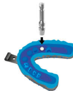
Reposition the coping, fixed onto the analog
