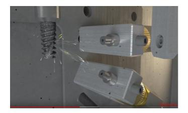
At the heart of the ST200 system is a revolutionary blasting technology, utilizing very small blasting nozzles, that produce focused and accurate high-pressure abrasive flow, producing excellent surface texturing, while Saving material, waste and money. During the blasting process, the robotic arm rotates and moves the implant in front of the blasting nozzles according to a user program, controlling the speed of rotation, feeds, travels, delays and sequences.
