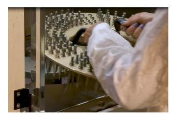
For more productivity, a set of interchangeable implants magazines is available as well as the AF108 system for used material recycling and automatic refill of the blasting media tanks.
