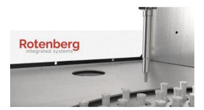
The implants are individually mounted on holders, creating a protective seal for the implant's platform.
