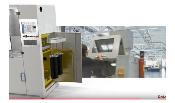
The ST200 programmable sandblaster is designed to work in the clean environment of medical fabrication facilities.
