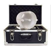
The CTDI Phantom Set consists of one 10 cm pediatric head phantom with five holes, one 16 cm head phantom adapter
