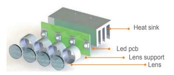
The optical system of Core White is made as shown in the figure. The light beams emitted by each of 4 LED sources are focused with special lenses and concentrated into one rectangular and homogeneous pattern. Special filters are used to eliminate I.R. on luminous pattern.
